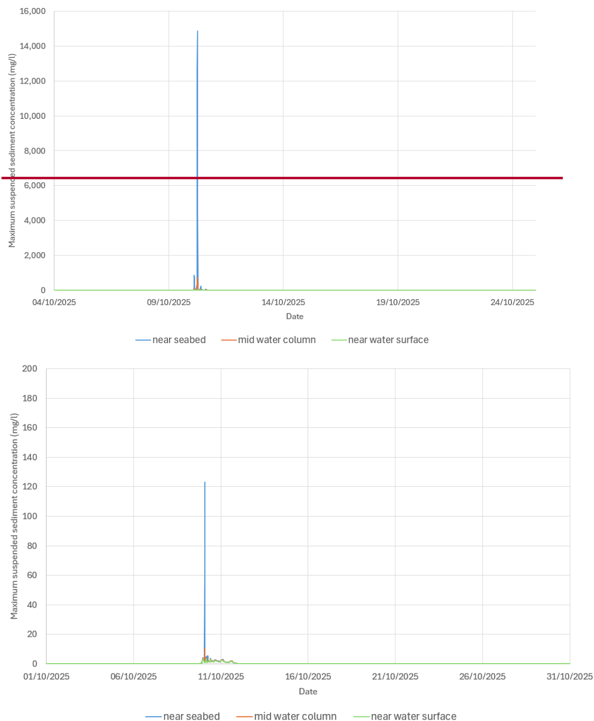
Figure 7.35 Time series of suspended sediment concentration at P2 during seabed preparation for array structures (smaller WTGs) near seabed, middle of water column and near water surface (array centre)
