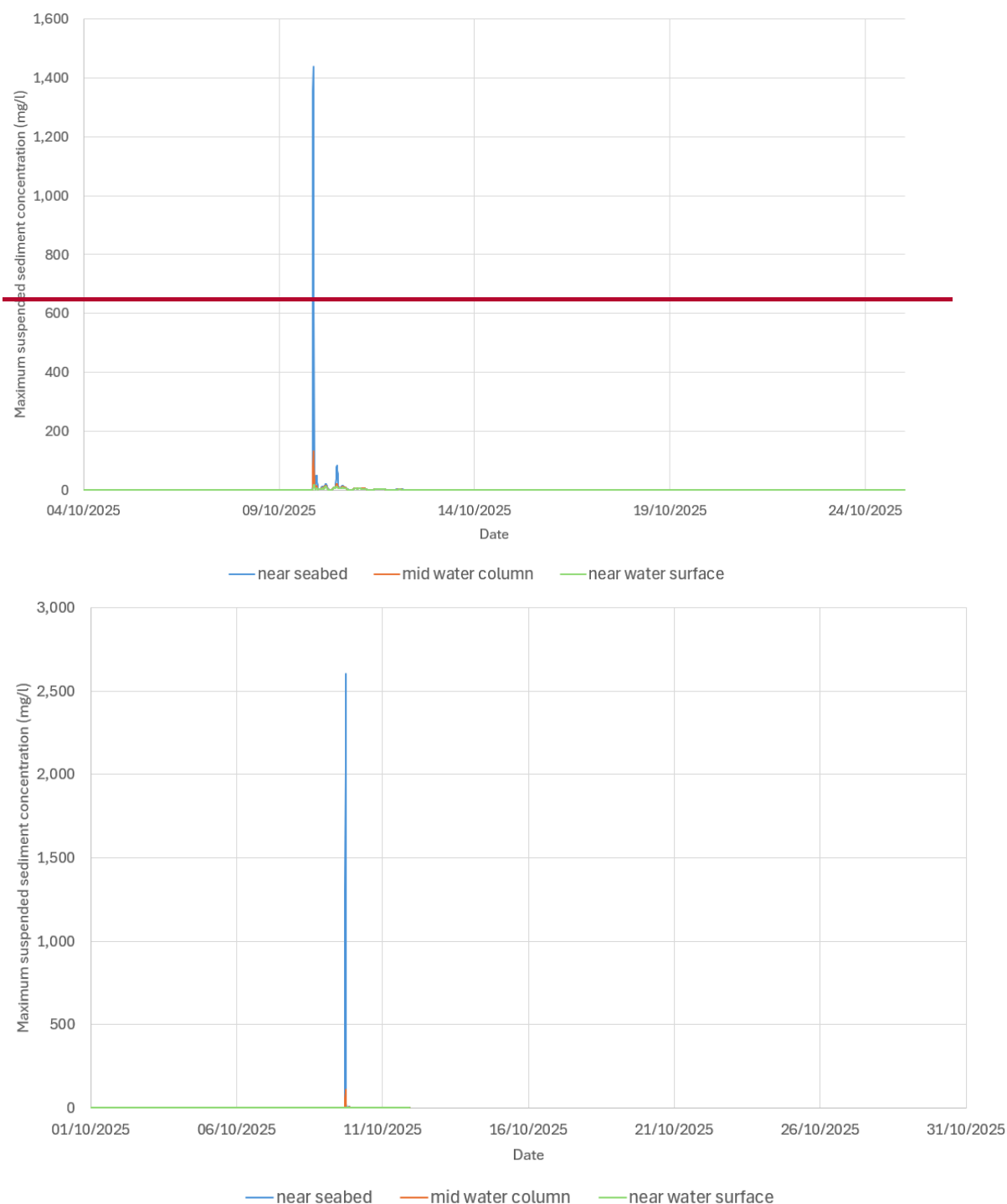
Figure 7.34 Time series of suspended sediment concentration at P1 during seabed preparation for array structures (smaller WTGs) near seabed, middle of water column and near water surface (near MCZ)
